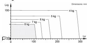
The KR 8 R1620 arc HW is designed for a rated payload of 8 kg in order to optimize the dynamic performance of the robot. With reduced load center distances, higher loads up to the maximum payload may be used. The specific load case must be verified using KUKA.Load. For further consultation, please contact KUKA Support.
