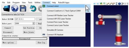
5. The following window will pop-up, change the robot IP according to the IP of your robot.
