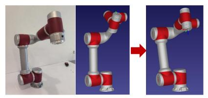
2. Move Joints will make the real Jaka Robot move to the position in RoboDK.
