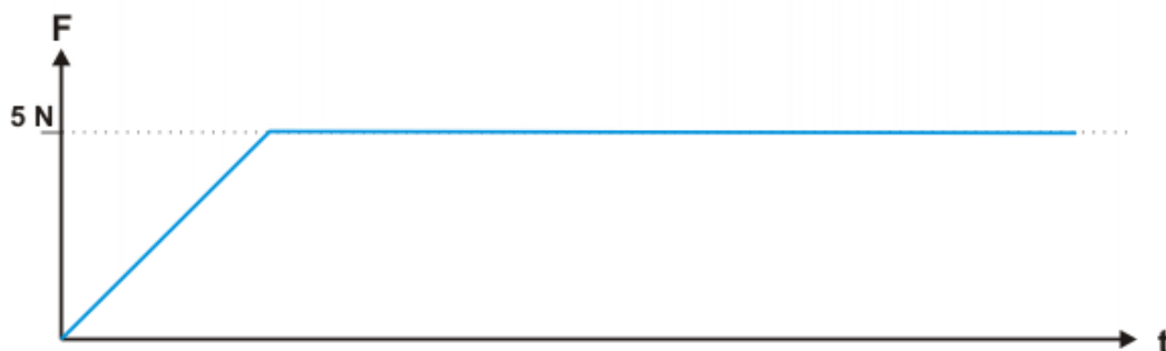
Force over time (high stiffness, small position difference)
